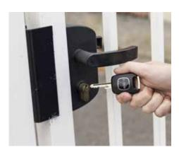
The new key transmits the information to the cylinder through an electromagnetic induction coil located at the heart of the key.
