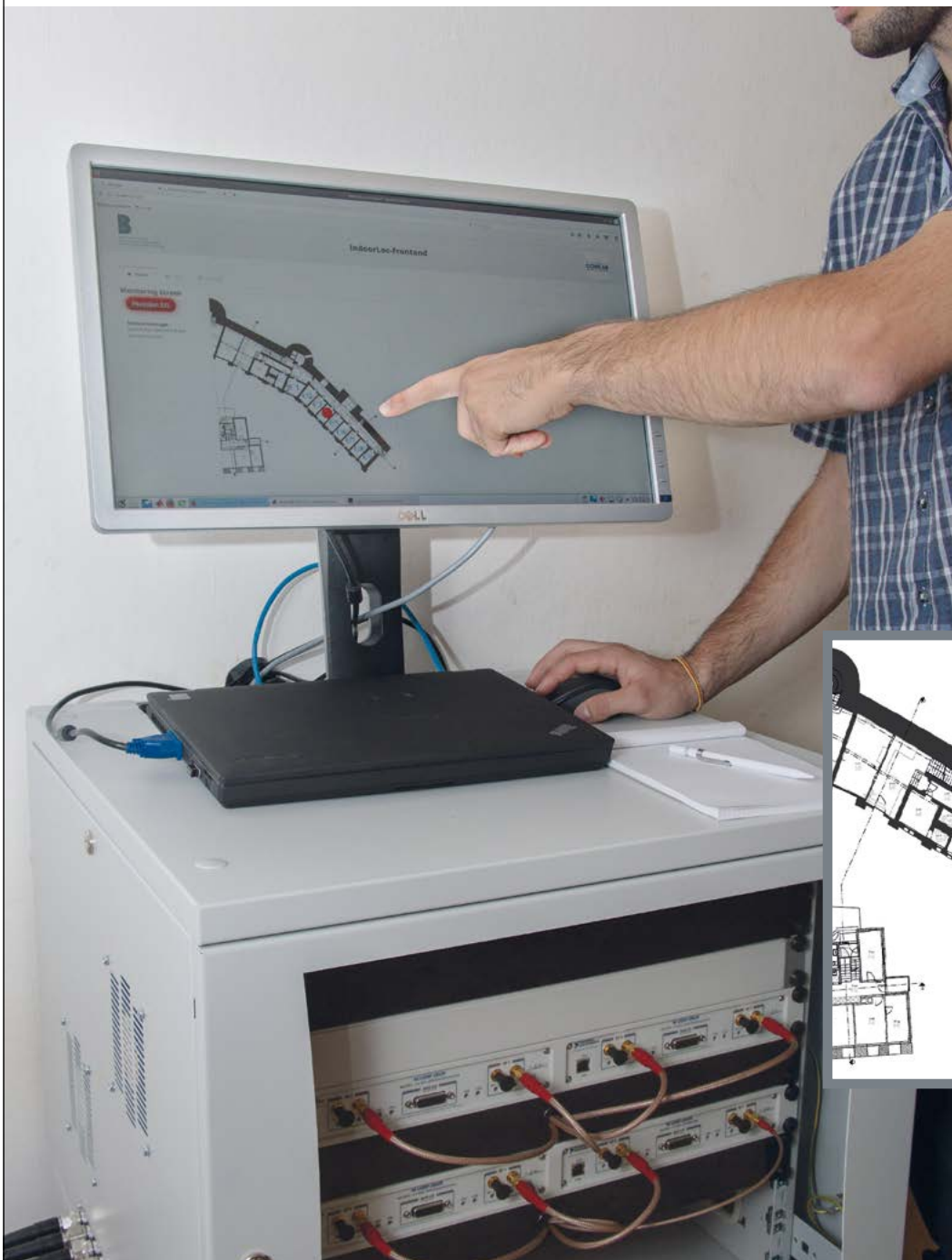
A prototype of the demonstration system developed by the University of Applied Sciences in Berne with active detection and localisation of smuggled mobile phones
