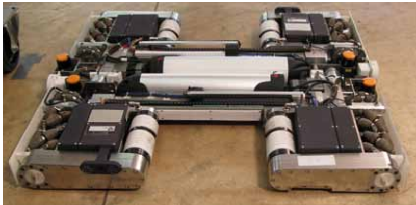
Working in pairs, the bogies position themselves under the vehicle before lifting its wheels on rollers
