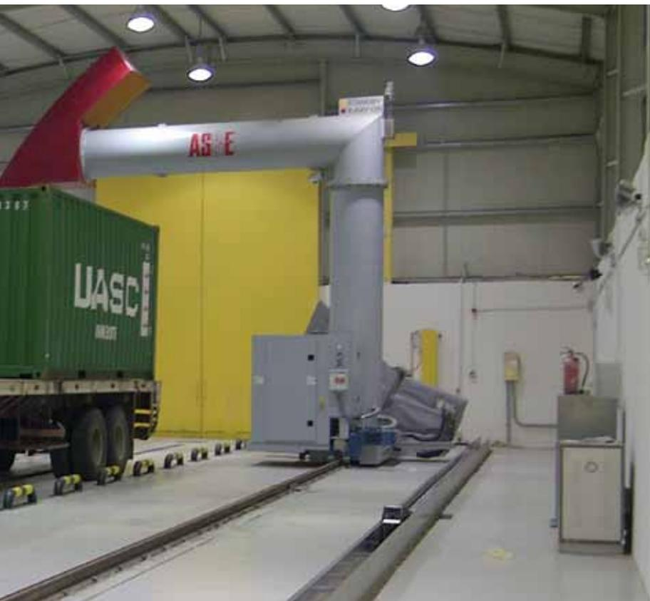
therefore use high-energy linear accelerators which emit significant amounts of radiation. Drivers and passengers must exit their vehicles and the scan tunnel prior to the scan to avoid exposure to excessive doses of radiation. The nature of gantry systems favours penetration and imaging performance over throughput.
